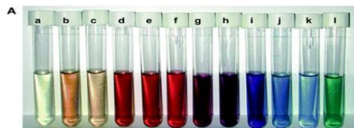
The change of color of colloidal solution depending on the size and shape of silver nanoparticles
