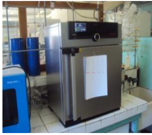
Photo-1 : Four Memmert programmable (photo labo)
